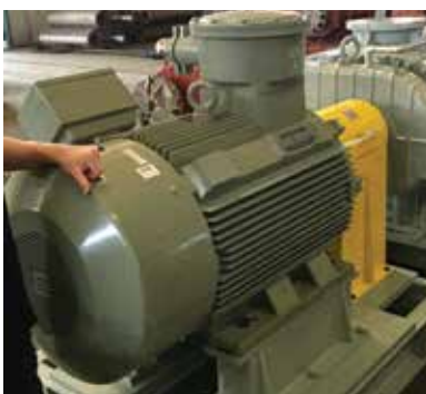
EXE 132 kW Roots high-pressure vacuum pump used in a High Vac project in NSW pharmaceutical plant
