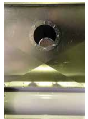
Removable Inspection window built into the hopper
