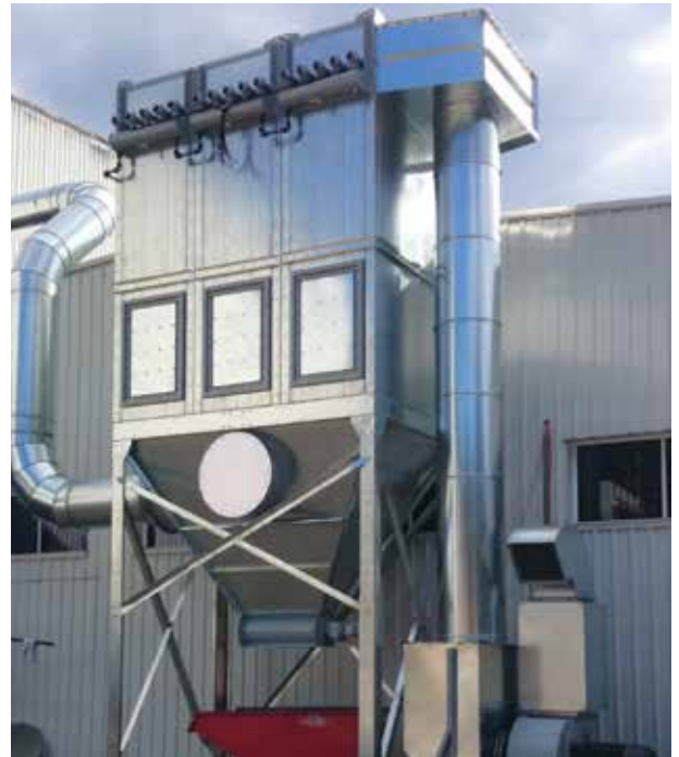
MDC36000P (45kW) , large saw dust application
