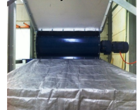
1 Mtr Rotary Valve feeds into a bin
