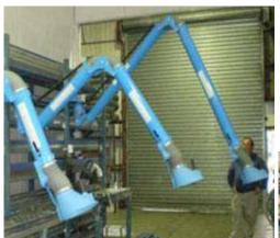
The Ezi-Duct Ezi-Arm is now available in 3 different sizes. Originally only available in 3.0 mtr model the
