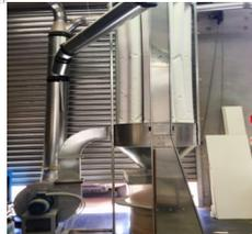
1 Mtr Rotary Valve feeds into a bin
